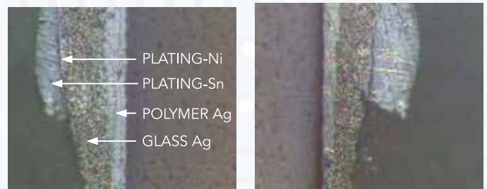
NO CRACKING APPARENT IN THE CERAMIC
